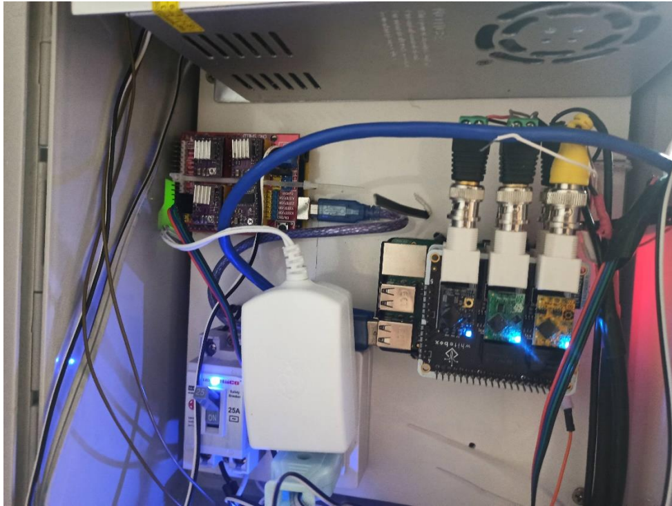
Figure 4.3 Box controller stepper motor and sensor
