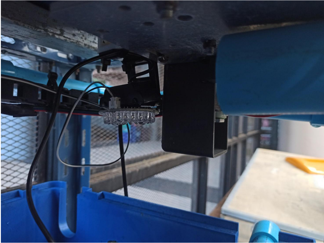
Figure 4.2 The overview of feeder and camera
