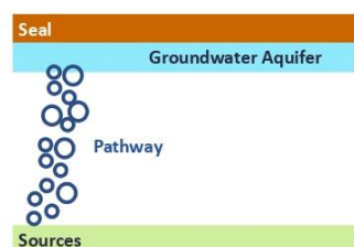
Fig. 1. Schematic drawing of the CO 2 pathway from various sources to be accumulated in groundwater becoming CO 2 -rich groundwater.
