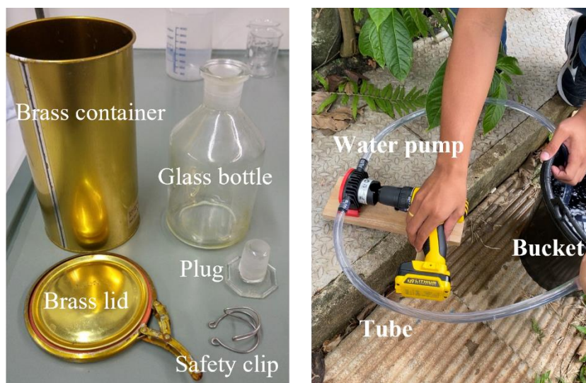
Figure 2.4 Water sampling container for CFC-SF 6 concentration analysis consists of five items: brass container with lid, glass bottle with plug and safety clip, water pump, tube and bucket.
