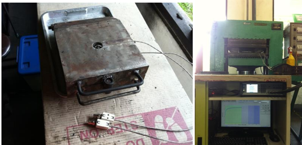
Figure 3.4 The embedded electrodes in compression mold and equipment settings.
