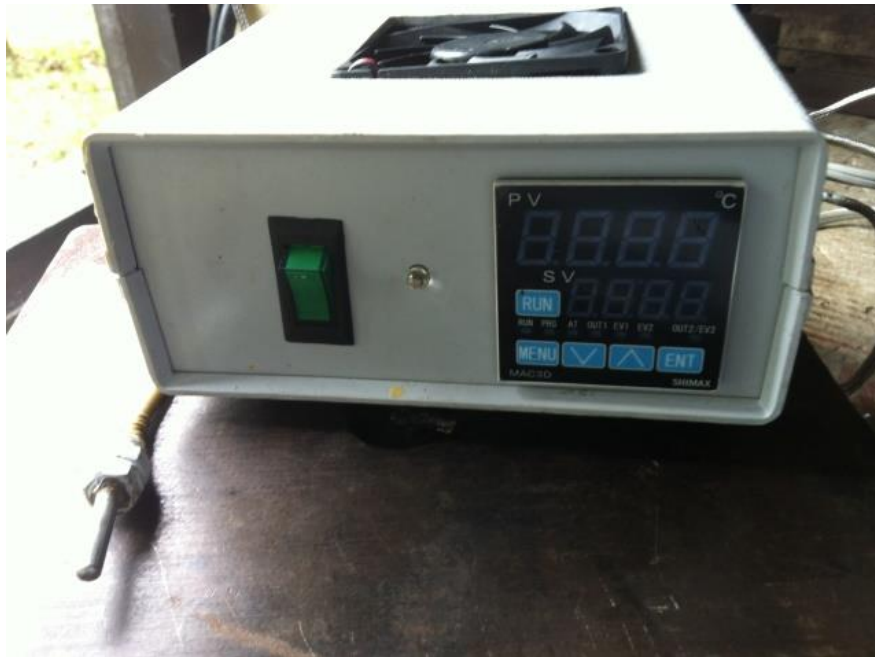
Figure 3.5 Thermocouples with a heat resistant strap and display unit.
