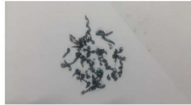
Fig. 5. Chips using cooking oil
