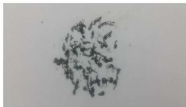
Fig. 6. Chips using olive oil
