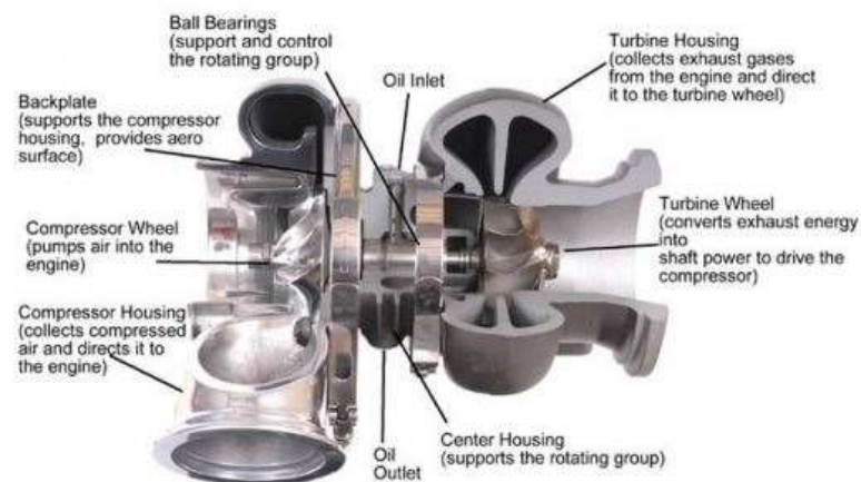
Figure 2.5: Typical Diagram of turbocharger (Kusztelan et al., 2011)
