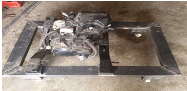
Figure 3.8: Engine Mounted on Frame
