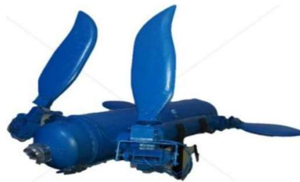
Fig. 2. UROV Assembly with Flappers
