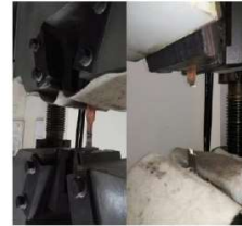
Figure 6 Tensile Testing on UTS MACHINE
