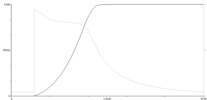
**Figure 3.16** Vestas V112-3.0 MW power curve
