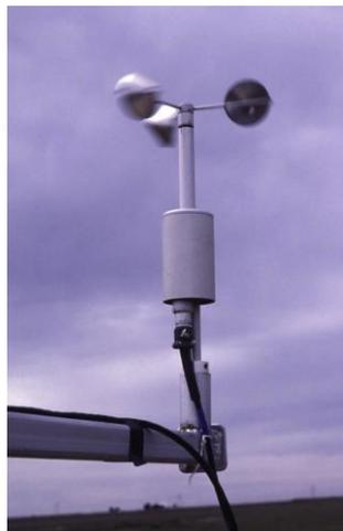
**Figure 2.2** Cup anemometer to measuring wind speed
