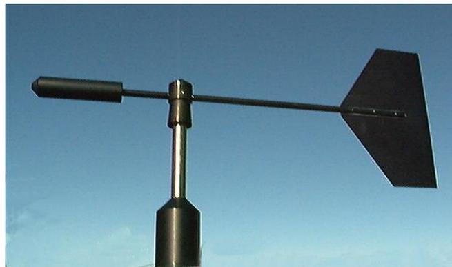
**Figure 2.1** Wind direction vane
