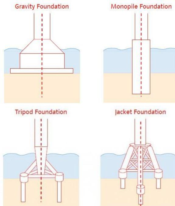
**Figure 2.7** Type of wind turbine foundation
