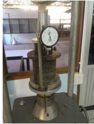
Fig. 8. Unconfined Compression Test.
