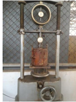
Fig. 6. California Bearing Ratio Test (CBR).
