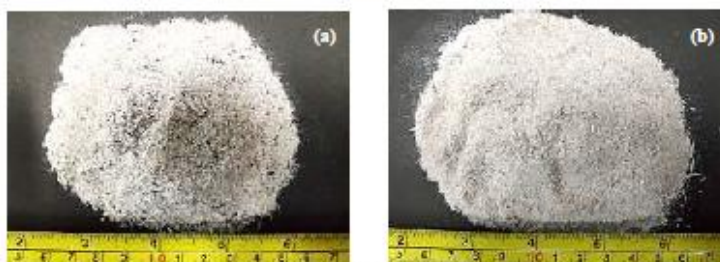
Figure 4: SYRHA after treatment processing of (a) open-air burned and (b) incinerated at 700 °C for 1 h
