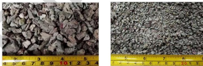
Figure 2 Crushed POBC Used as (a) Coarse Aggregate (POBCCA) and (b) Fine Aggregate (POBCFA)
