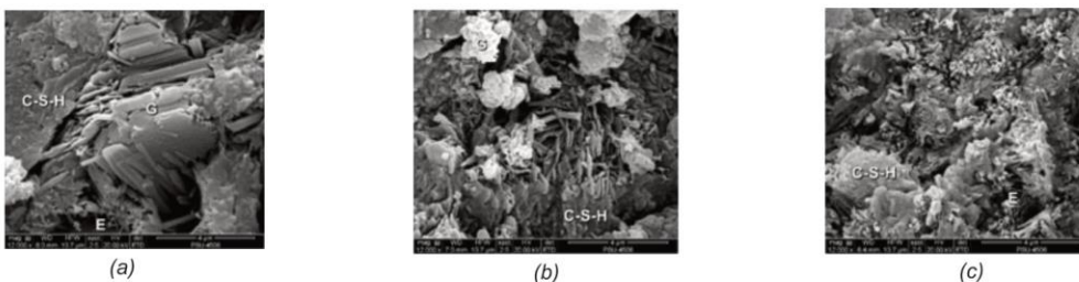
Figure 11: Scanning electron micrographs of the 56-day OPC specimen (a), specimen incorporating 10% RHA (b), and 10% CB (c) after exposure to sulphuric acid solution for 42 days
