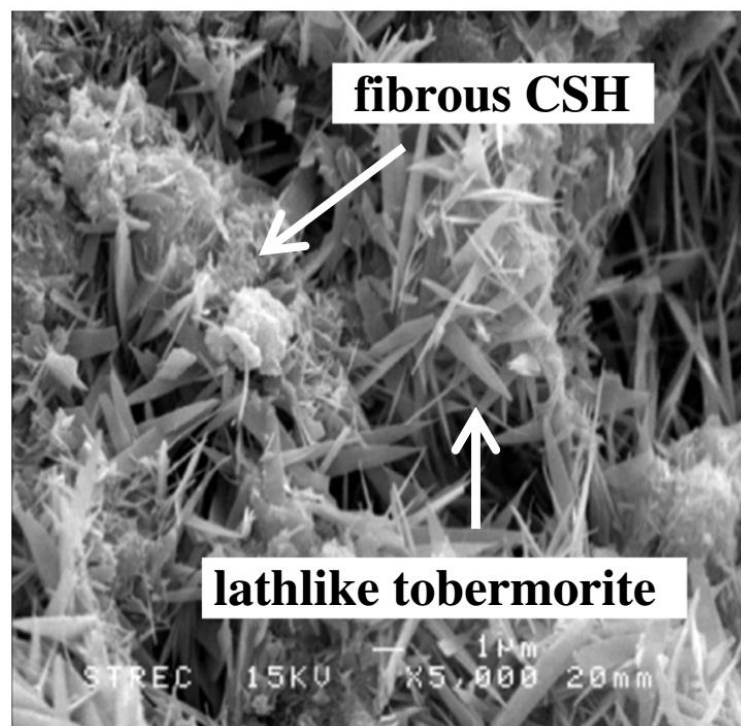
Figure 4 SEM image of autoclaved aerated concrete containing RHA and aluminum powder (Kunchariyakun et al., 2015)
