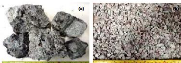
Figure 2: POBC sample (a) lumps and (b) aggregate used
