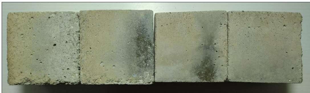
Figure 24 Visual observation of deteriorating characteristics of POBC mortars exposed to sulfuric acid solution for 42 days (from left to right: control mix, R10, R20, and R30)
