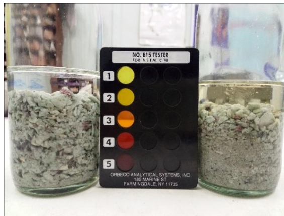
Figure 9 The organic impurity test of POBC aggregate as per ASTM C40
