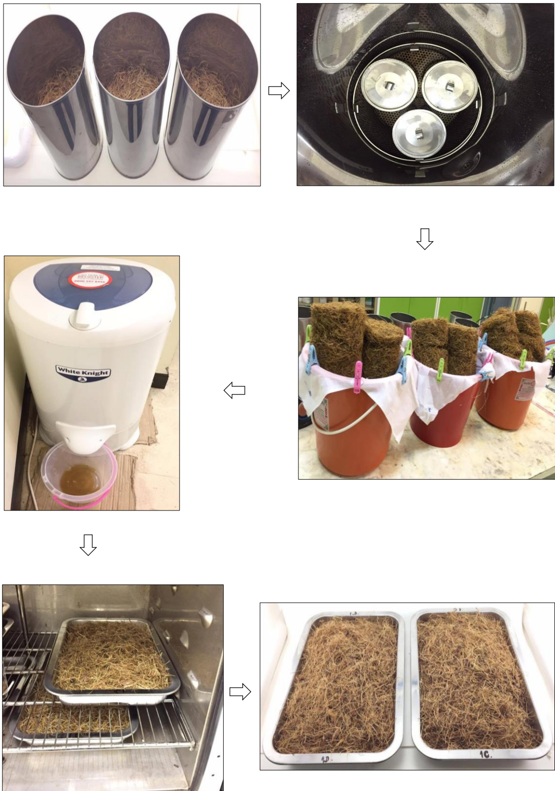
Fig. 3 Brief process of hydrothermal treatment to final dried EFB sample.
