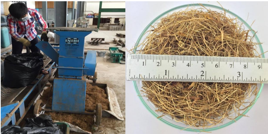
Fig. 2 Shredding palm empty fruit bunch into 2-5 cm.
