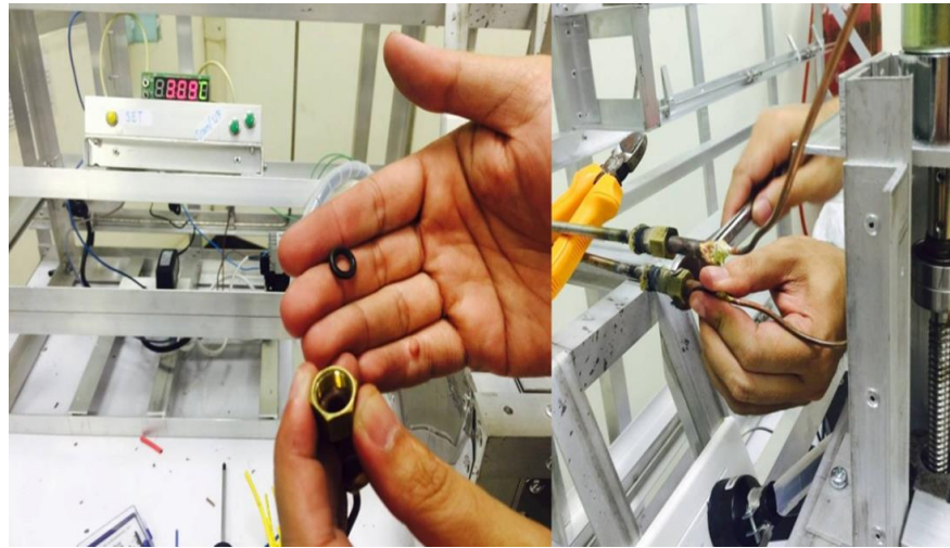
Figure 3.58. Installation of O-rings in the mating surface pipes/valves in Solid oxide fuel cell testing system.
