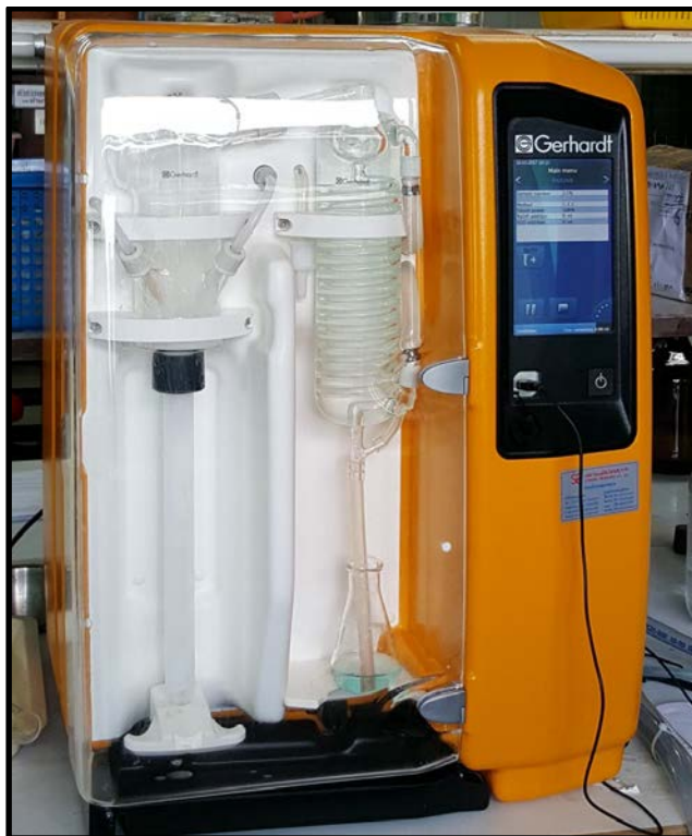
Figure 3.5 Apparatus for distillation system.
