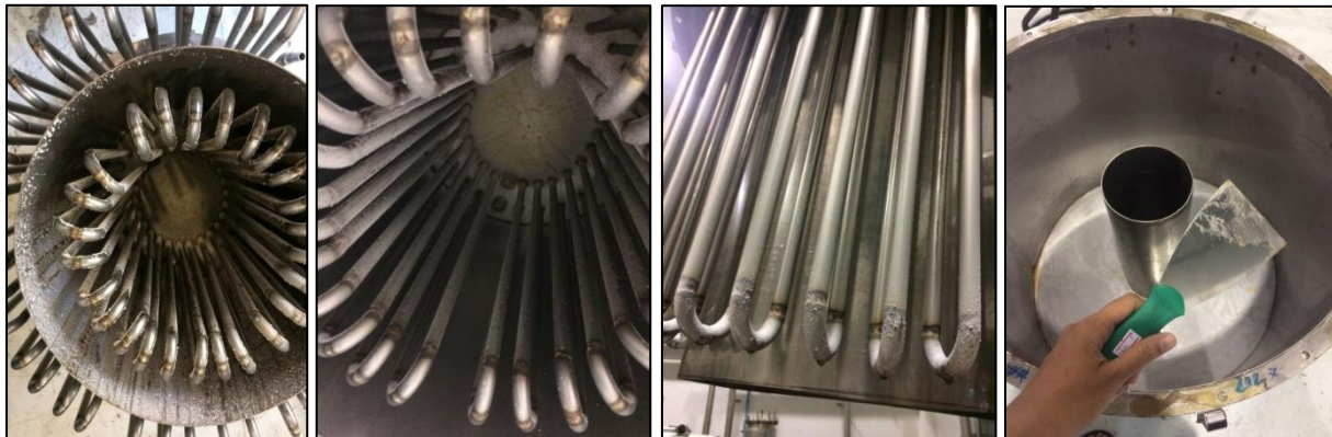
Figure 4 Structure of internal free fatty acid separation reactor.
