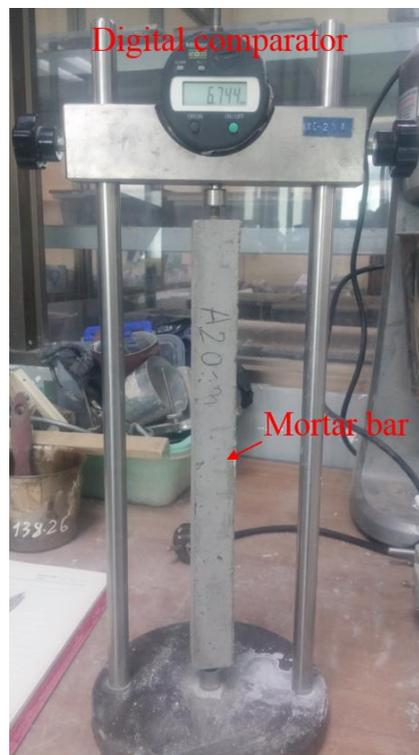
Figure 16. Record the comparator reading of the specimen
