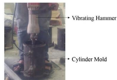
Fig. 5. The 150 × 300 mm cylinder mold and vibrating hammer.
