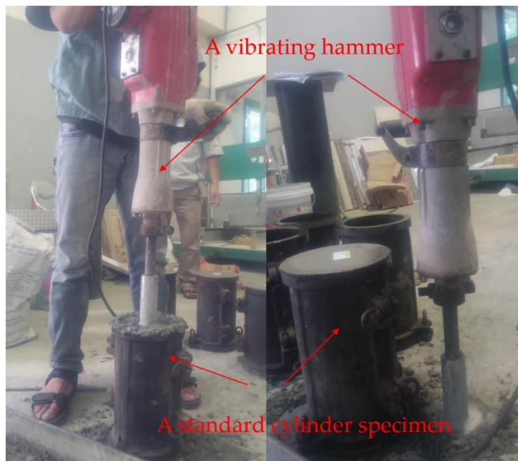
Figure 12. The 150 x 300 mm cylinder specimen and the vibrating hammer
