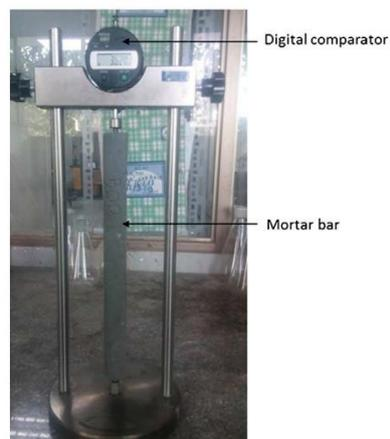
Fig. 4. Record the comparator reading of the specimen.
