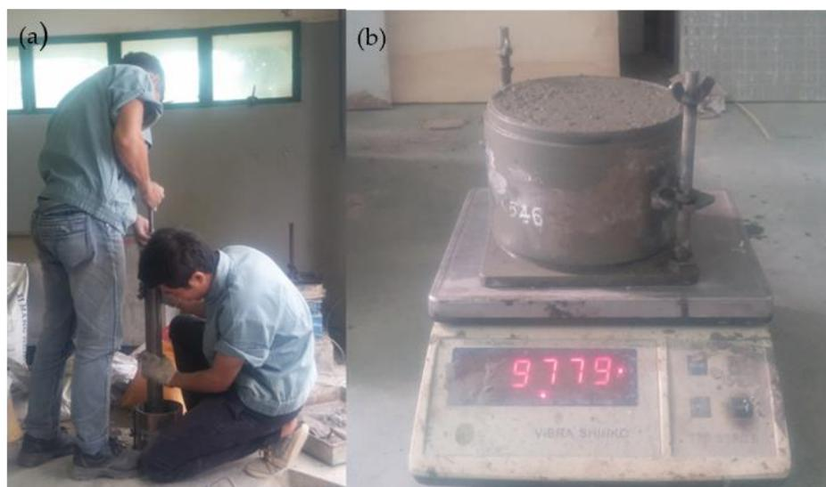
**Figure II.** Proctor test, (a) compacting the mixture in the mold, (b) determining the density of mixture after compacting.
