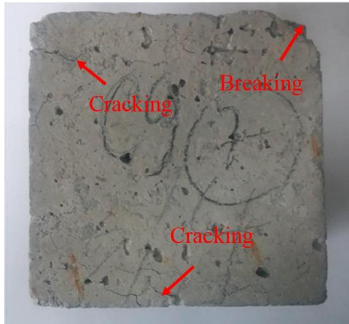
Figure 38. Cracking image of C40's sample exposed to sulfate environment 8 weeks
