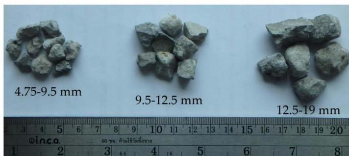
Figure 1. Electric arc furnace (EAF) slag aggregate used in this study.
