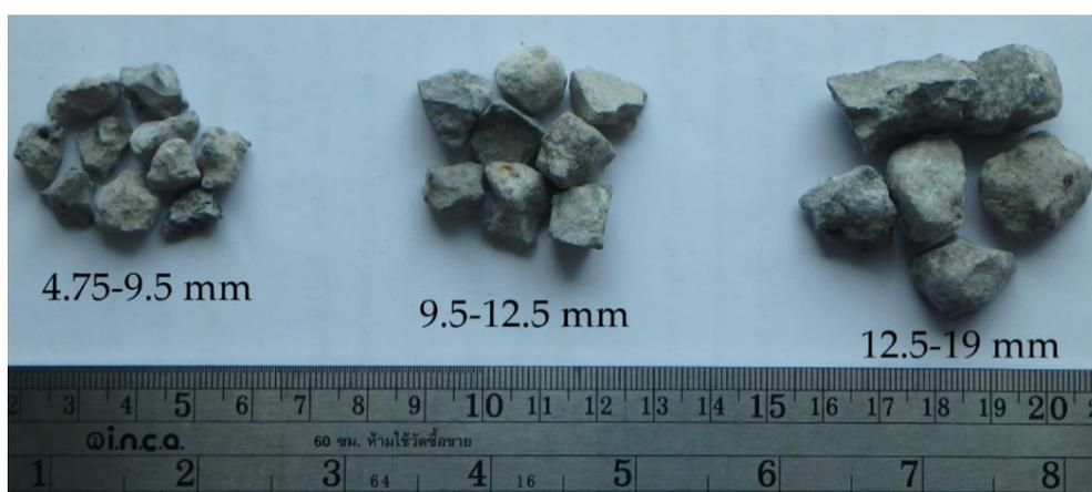
Figure 8. EAF slag aggregate used in this study
