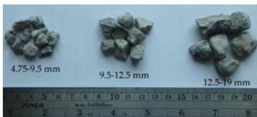
**Figure I.** EAF slag aggregate used in this study.
