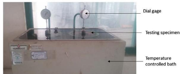
Fig. 3. The testing specimens were stored in water at  $70 \pm 3$  °C.
