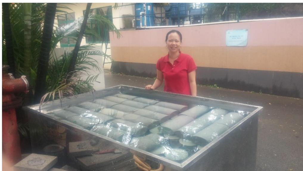
Figure 13. The curing of specimens in tap water
