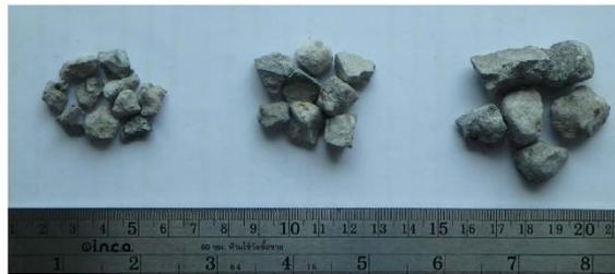
Fig. 2. Three particle sizes (i.e. 4.75–9.5 mm, 9.5–12.5 mm and 12.5–19 mm) of EAF slag aggregate used in this study.
