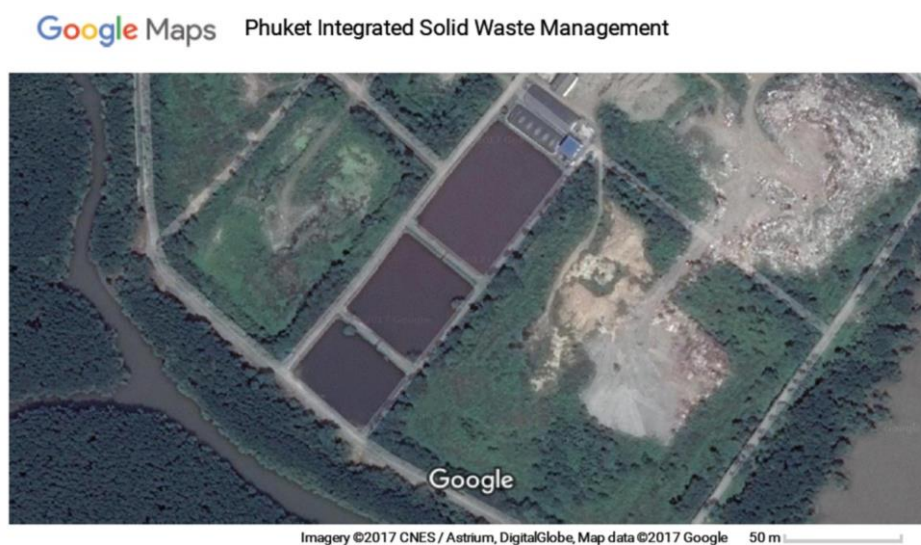
Figure 6 Sewage Ponds at Phuket Waste Management. The Central Pond is at Lat 7.860077, Long 98.391960. The red colour is due to Rhodospseudomonad photosynthetic bacteria although green algae are also present.
