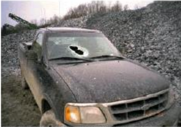
1. Fatal injury due to flyrock at a limestone mine in Pennsylvania (Case Study No.6) Source: MSHA, 1999b
