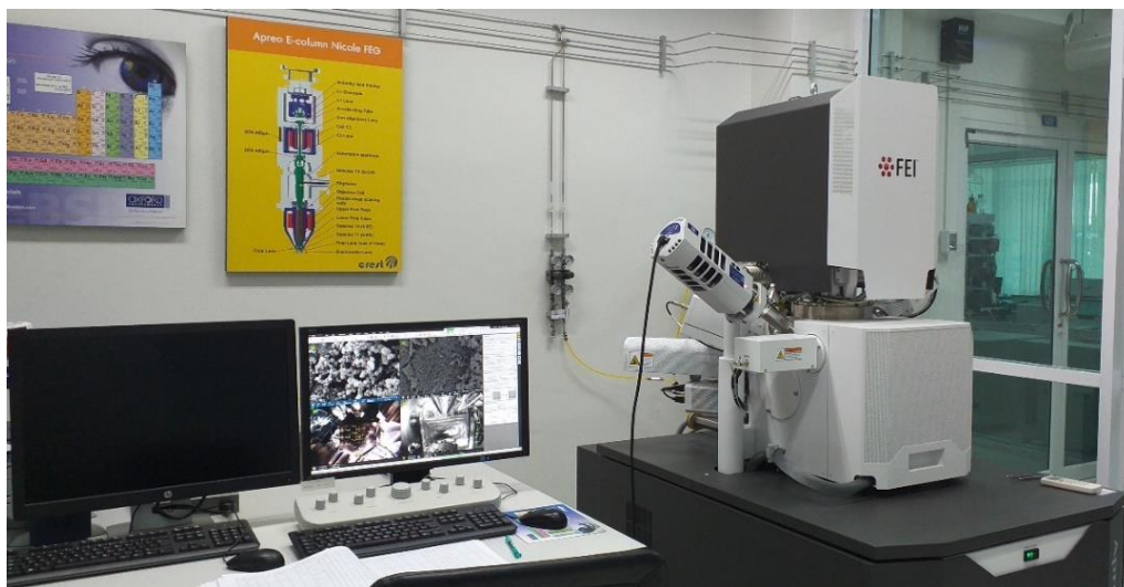
Figure 2.22. Real picture of scanning electron microscope (FE-SEM; FEI Quanta-400, Czech Republic), scientist equipment center (SEC) in Prince of Songkla University.
