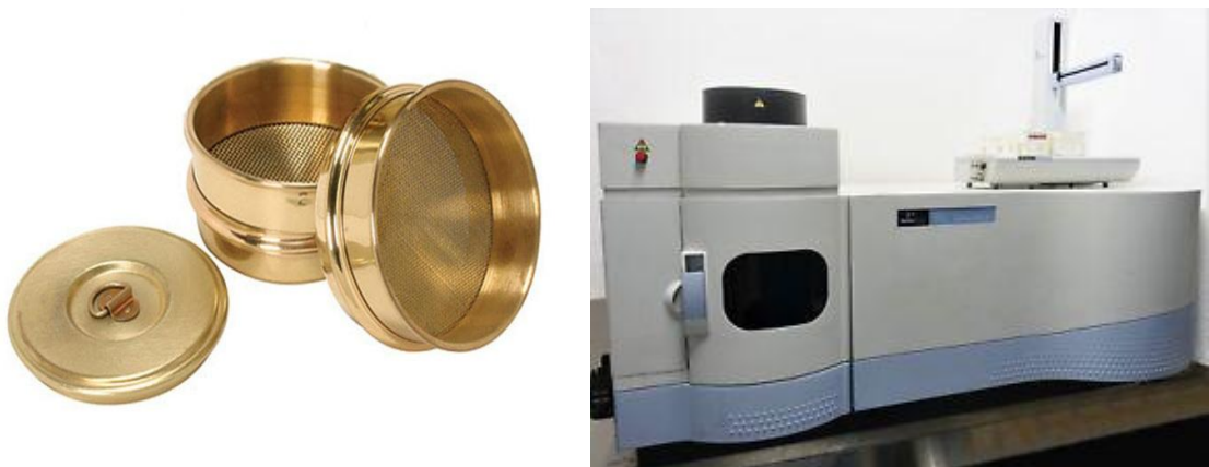
Figure 3.13 Soils analysis equipments (sieves, Perkin Elmer Optima, 4300 DV/Perkin Elmer Optima 800)
