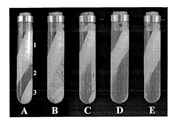
Figure 9 Fractionation by centrifugation of fresh *Hevea* latex (45,000 x g from centrifuge model L8-70M, Beckman). A: freshly tapped latex (0 time); B: after standing at room temperature for 45 min; C: 60 min; D: 90 min; E: 120 min.
