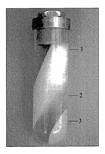
Figure 1 Fractionation of fresh *Hevea* rubber latex by untracentrifugation into three major zones. (1: rubber layer, 2: C-serum, 3: bottom fraction)
