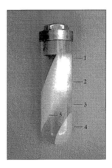
Figure 8 Ultracentrifuged fresh latex (45,000 x g from centrifuge model L8-70M, Beckman). 1: top layer consist of white and creamy rubber layer, 2: the yellow orange layer which was Frey-Wyssling membrane debris, 3: a clear solution called C-serum, 4: yellowish bottom fraction, and 5: zone 2 rubber.
