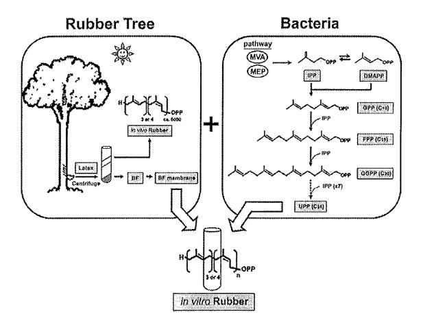
Figure 34 Schematic view proposing the interactive combinations of plant and bacteria in rubber biosynthesis
