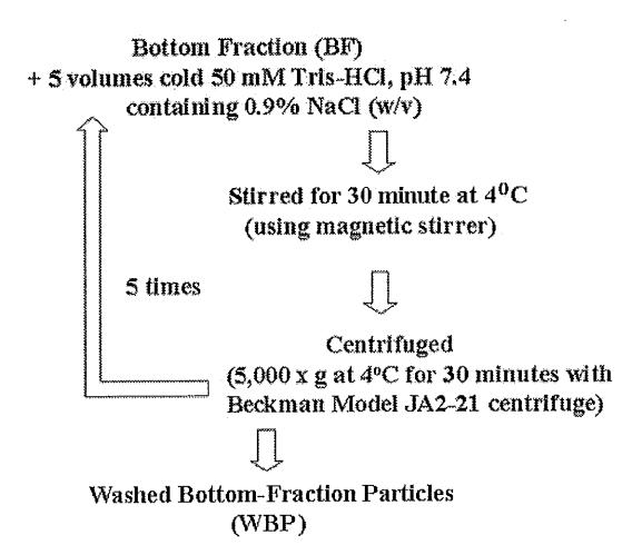
Figure 5 Summarized diagram for wash bottom-fraction particles (WBP) preparation.
