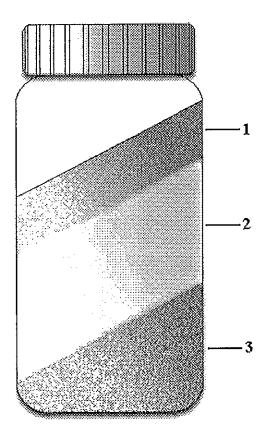
Figure 4 The centrifuged fresh latex (5,000 x g from centrifuge model JA2-21, Beckman). 1: top zone consist of white and creamy rubber layer), 2: aqueous middle zone containing C-serum and 3: yellowish at the bottom of the bottle called "Bottom fraction (BF)" containing membrane bound organelles, lutoid and Frey-Wyssling particles.
