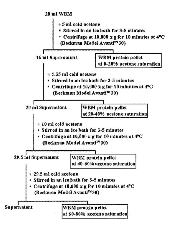
Figure 7 Summarized diagram for serial acetone fractionation of WBM proteins.
