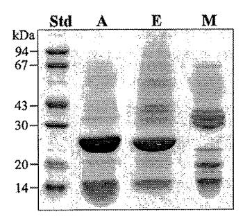
Figure 10 SDS-PAGE analyses of proteins extracted from different fractions of Hevea latex. A: proteins from RP of freshly tapped latex (Figure 9, tube A); E: proteins from RP of the delayed use latex (Figure 9, tube E); M: proteins from WBM prepared from freshly tapped latex (Figure 9, tube A); Std: standard molecular weight proteins.
