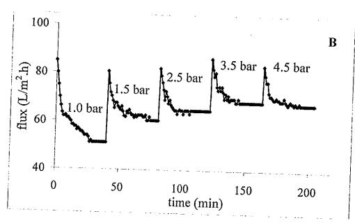
Figure 19 Flux vs. time during UF using with MWCO 30 kDa (A) and 100 kDa (B) regenerated cellulose membranes with cross flow rate 360 L/h at room temperature (30°C)
