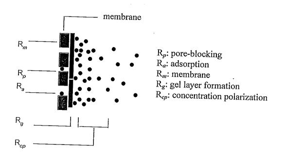
Figure 3 Possible resistances against solvent transport during UF Source: Berg and Smolders (1990)
