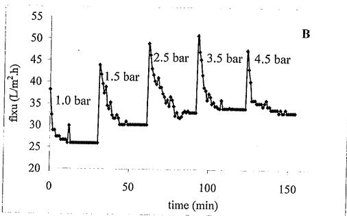
Figure 17 Flux vs. time during UF using MWCO 30 kDa (A) and 100 kDa (B) regenerated cellulose membranes with cross flow rate 120 L/h at room temperature (30°C)
