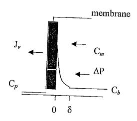
Figure 6. The concentration profile according to the film theory ( $\Delta P$ : transmembrane pressure;  $C_m$ , the concentration at the membrane interface;  $C_b$ , the concentration in bulk;  $C_p$ , the concentration in the permeate; D, diffusion coefficient;  $\delta$ : thickness of the boundary layer)
