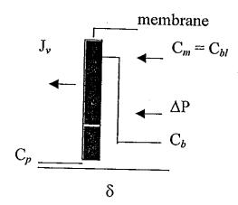
Figure 5 The cake-filtration type of description ( $\Delta P$ : transmembrane pressure;  $C_m$ : concentration at the membrane interface;  $C_{bl}$ : constant concentration in the boundary layer;  $\delta$ : thickness of the boundary layer)
