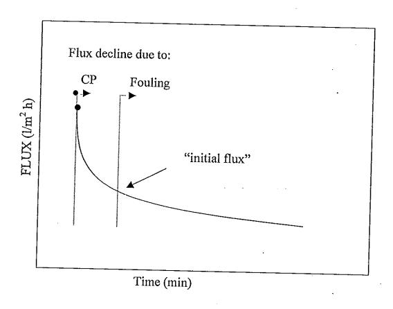
Figure 4 Flux decline is caused by concentration polarization (CP) and fouling. The pure water flux is indicated by (•)
