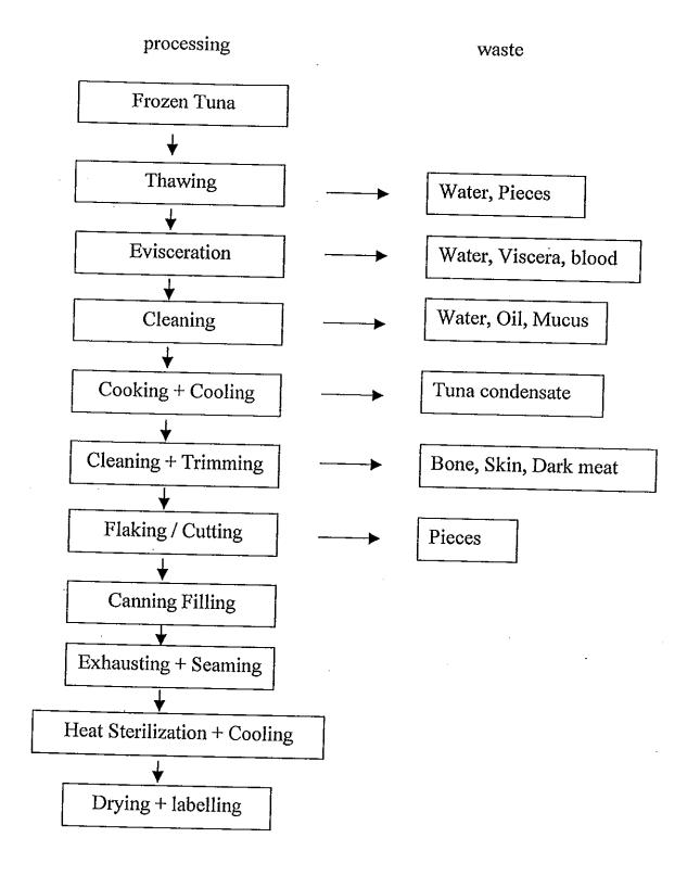
Figure 8 Typical flow-chart for the canning of tuna Source: H-Kittikun (2003)
