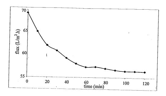
Figure 21 Flux vs. time during continuous DF for extract of tuna spleen by regenerated cellulose membrane with MWCO 30 kDa using cross flow rate 360 L/h and TMP 1.5 bar at  $30^{\circ}$ C
