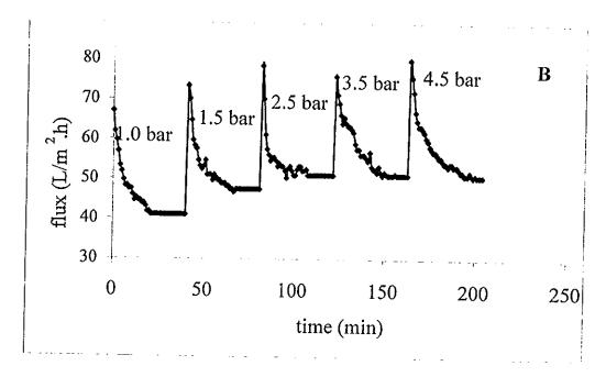
Figure 18 Flux vs. time during UF using MWCO 30 kDa (A) and 100 kDa (B) regenerated cellulose membranes with cross flow rate 240 L/h at room temperature (30°C)
