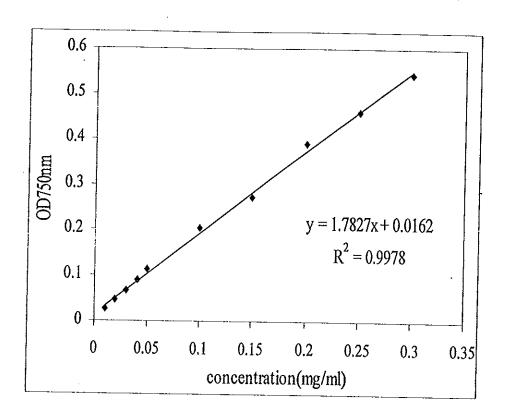
Figure-Appendix B1 Standard curve of BSA at the absorbance of 750 nm
