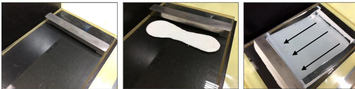
Figure 3.9 Casting procedure and equipment used to prepare the films in this study.
