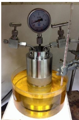
Figure 3.2 The high pressure reactor used in this study.
