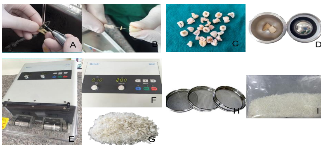
Figure 1 Demonstration of the human teeth milling process; tooth section (A-C), tooth milling (C-G) and particle size selection (H, I)
