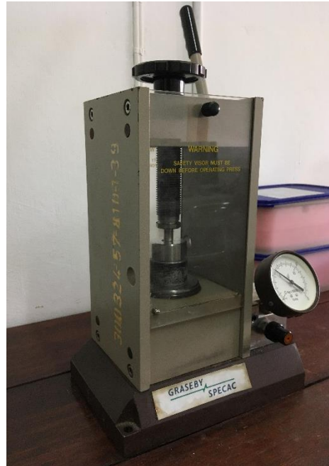
Figure 3.2 Pellet preparation tool in the process of preparing closely-packed sample.
