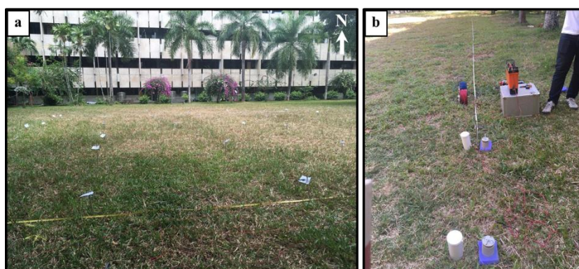
Figure 2.12 (a) Testing area at Science courtyard of Prince of Songkla University, (b) efficiency tests of Pb/PbCl 2 non-polarizing electrodes.
