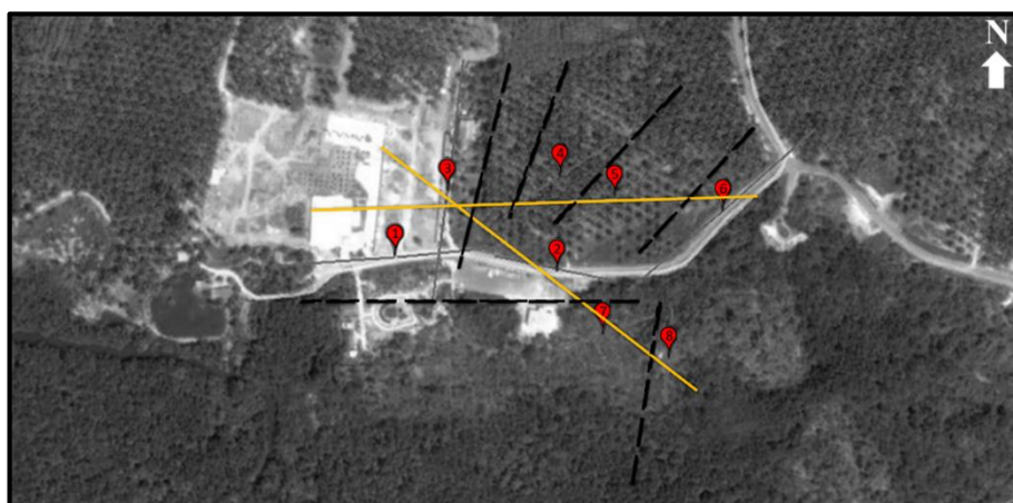
Figure 4.11 Location of cross section 1 and 2, and the assumed location of possible faults or fracture base on the combination of self-potential with VES.
