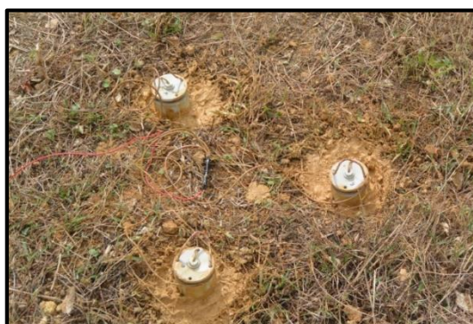
Figure 2.10 Three non-polarizing electrodes in holes and connected as base station; they were buried 30 cm from each other to evaluate the self-potential error related with this particular base station.
