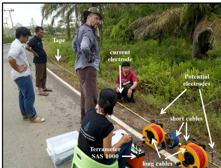
Figure 2.16 Basic equipment for VES measurement, Terrameter SAS 1000 connected by cables to steel electrodes.
