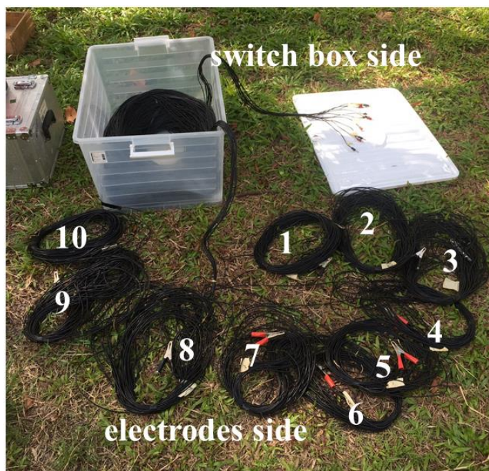
Figure 2.2 Cable assembly consists of ten single cables assembled together.
