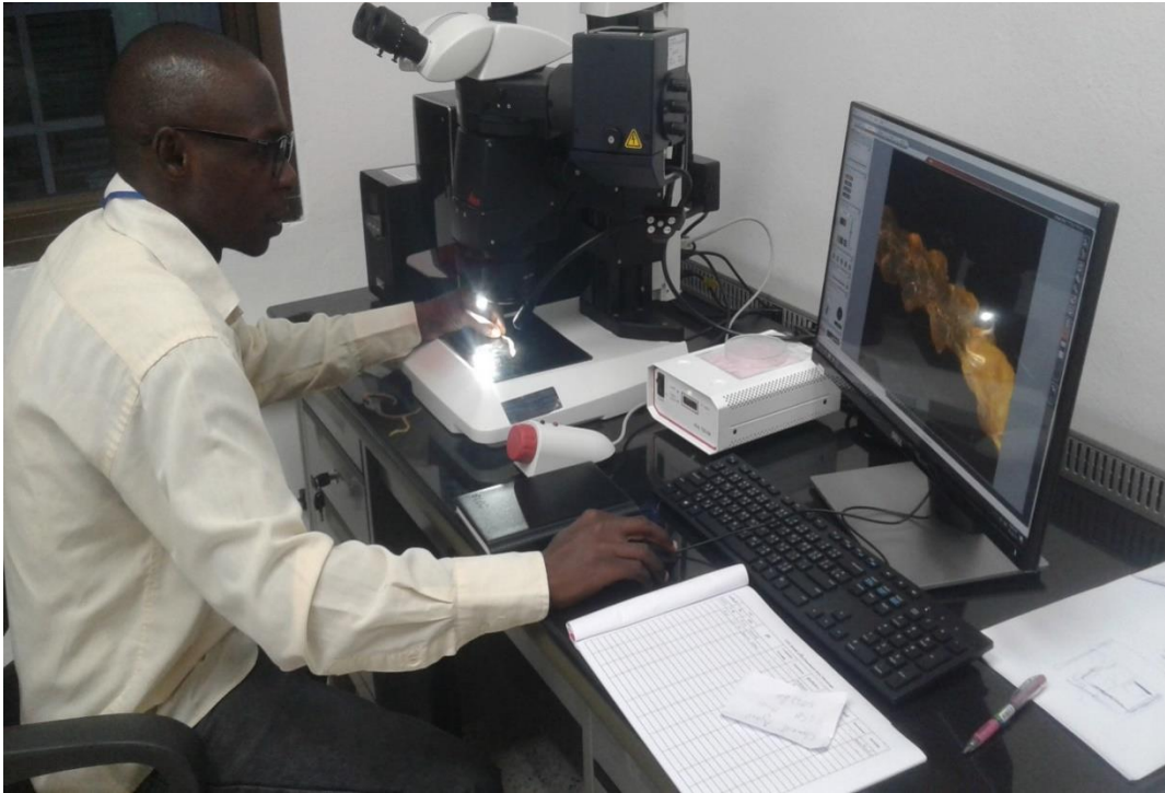
Plate A1: CLSM scanning and measurement of rubber sheet thickness.
