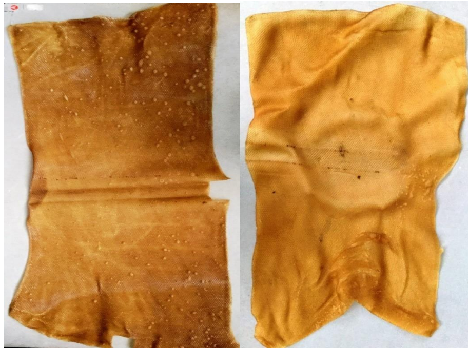
Figure 4.27 Rubber sheets with bubbles formed at 4.0 m/s, 40% RH and 65°C.
