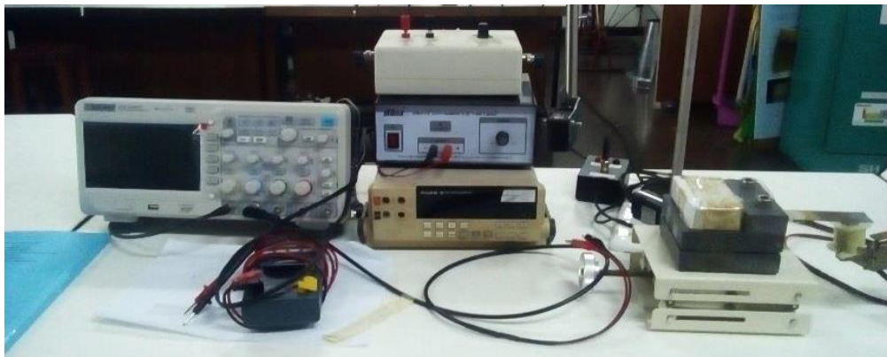
Figure 4.9 Vibrational piezoelectric generator experiments setup.
