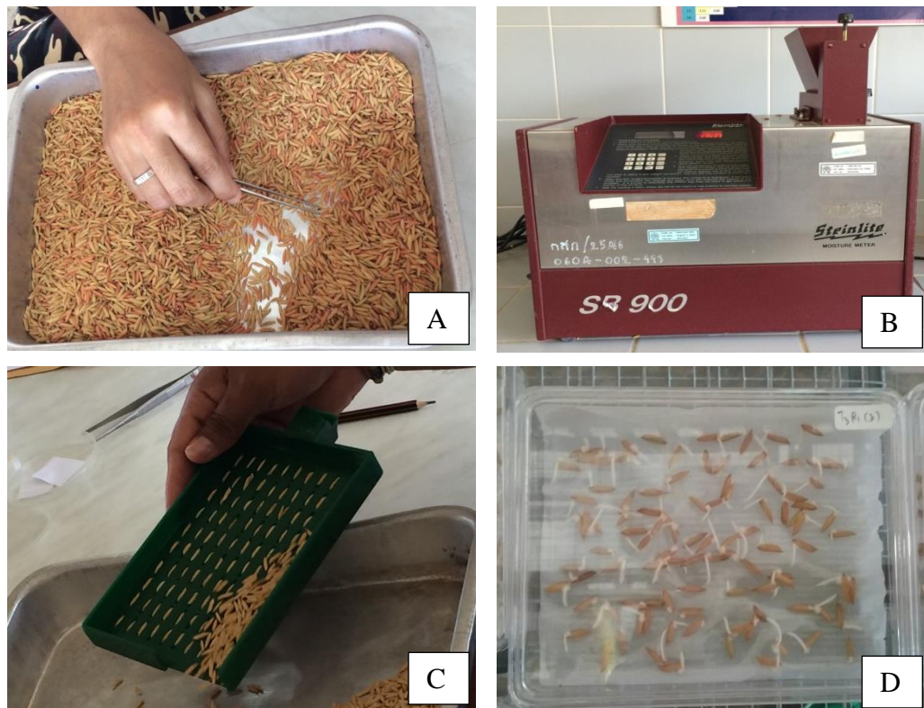
Figure 15 Counting number of insect (A), measuring moisture content through grain moisture meter (B) and test of seed germination (C and D).
