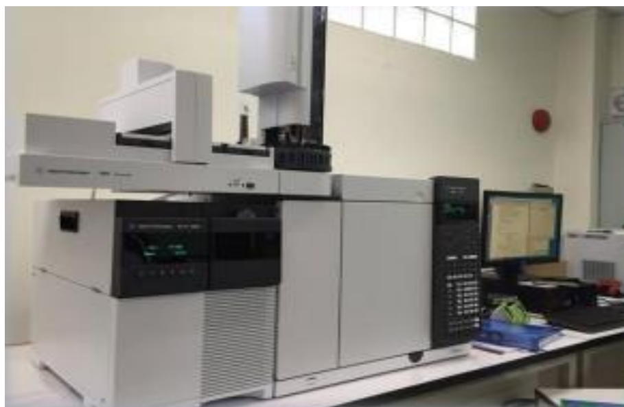
Figure 10 Gas Chromatography-Mass Spectrometry (GC-MS 7890B GC-5977 A MSD, Agilent, USA) used for chemical composition and quantification.
