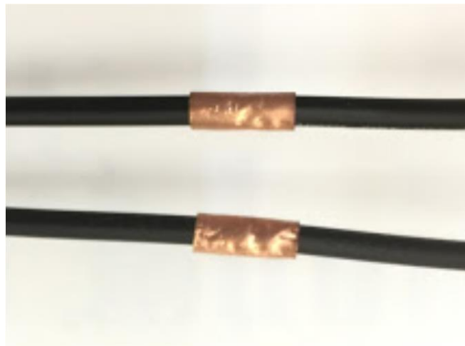
Figure D.2: The capacitive sensors wrapped on cables
