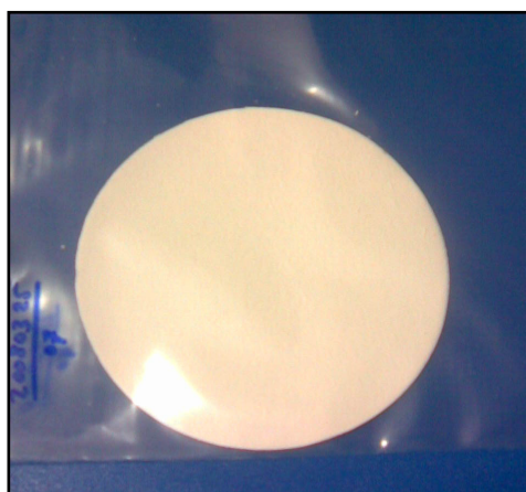
Figure 3.7 Photograph of a quartz fiber filter (ADVANTEC, QR-100) with 110-mm-diameter.
