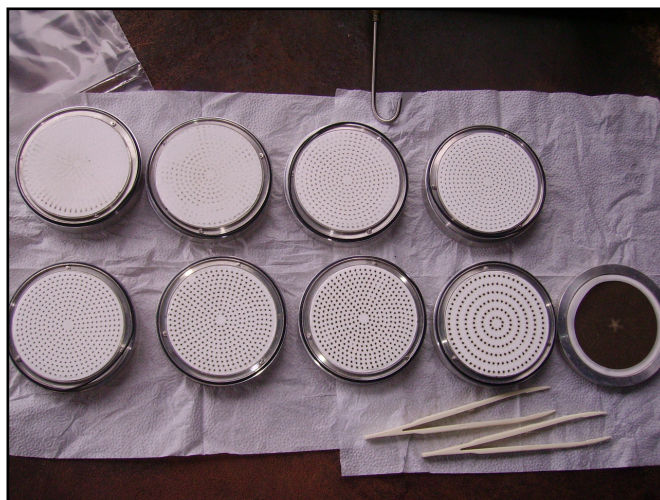
Figure 3.14. Photograph of filters of each stage after sampling with Andersen sampler.
