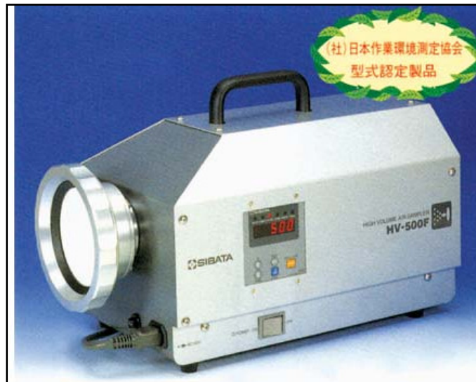
Figure 3.8 Photograph of the high volume sampler (Sibata, HV500F) used for measuring the total suspension particulate matters.
