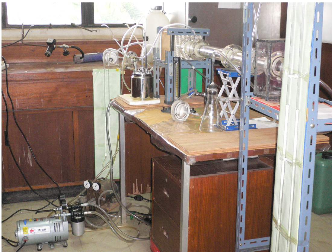
Figure 3.8 Photograph of the experimental set-up for studying the collection characteristics of mist aerosol particles.
