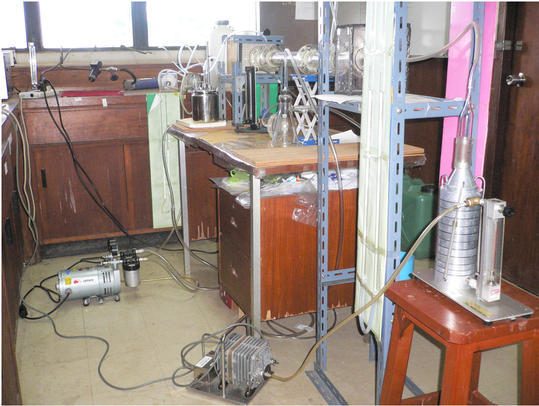
Figure 3.2 Photograph of the experimental set-up for examining size distribution and stability of generated aerosol.
