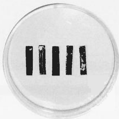
Figure 3.11 Thin film gold electrodes fabricating by thermal evaporation technique.
