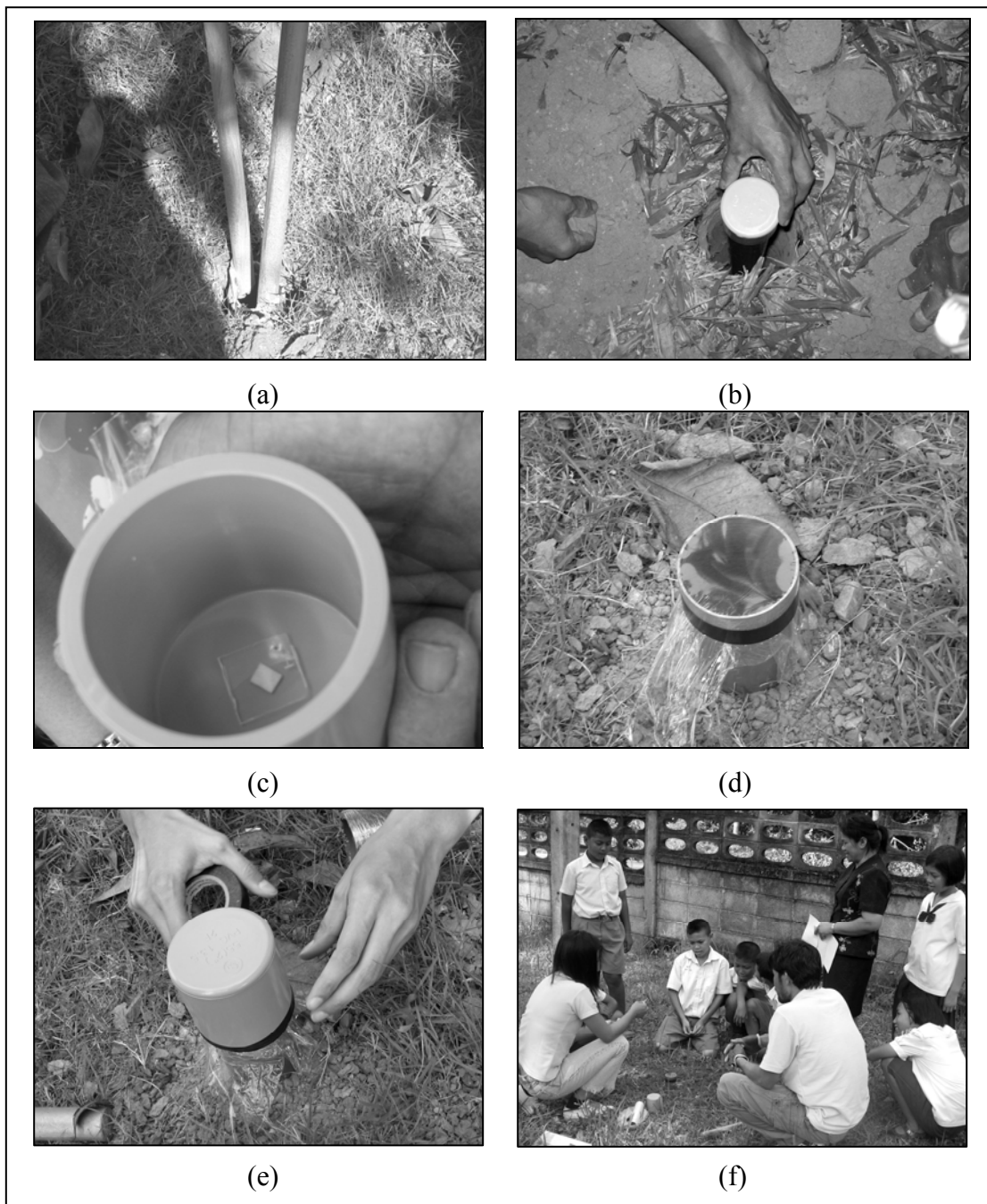
Figure 2.7 The measurement method of track detector for radon in soil gas: (a) a hole of 1 m depth, (b) a plastic tube put into the hole, (c) the tube was covered with thin polyethylene film and sealed airtight by a standard electrical tape, (d) the CR-39 film in a lid, (e) cover tube lid down and sealed airtight by a standard electrical tape, and (f) CR-39 film was changed every week.
