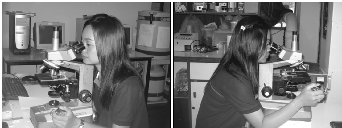
Figure 2.3 Counting tracks by using an optical microscope (OLYMPUS-BHC) at magnifications 10 \times 10 ( \times 100 ).
