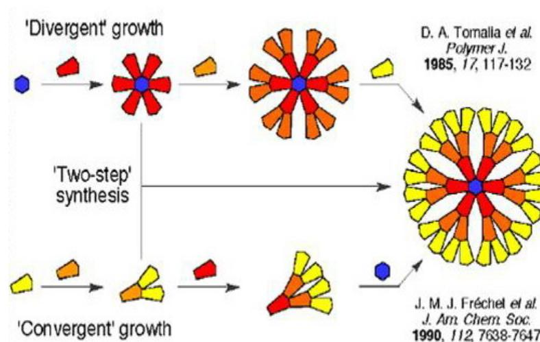
**Figure 1.5** Dendrimer synthesis approaches: divergent synthesis and convergent synthesis (from <http://www.eng.buffalo.edu/Courses/ce435/Dendrimers/Dendrimers.html>).
