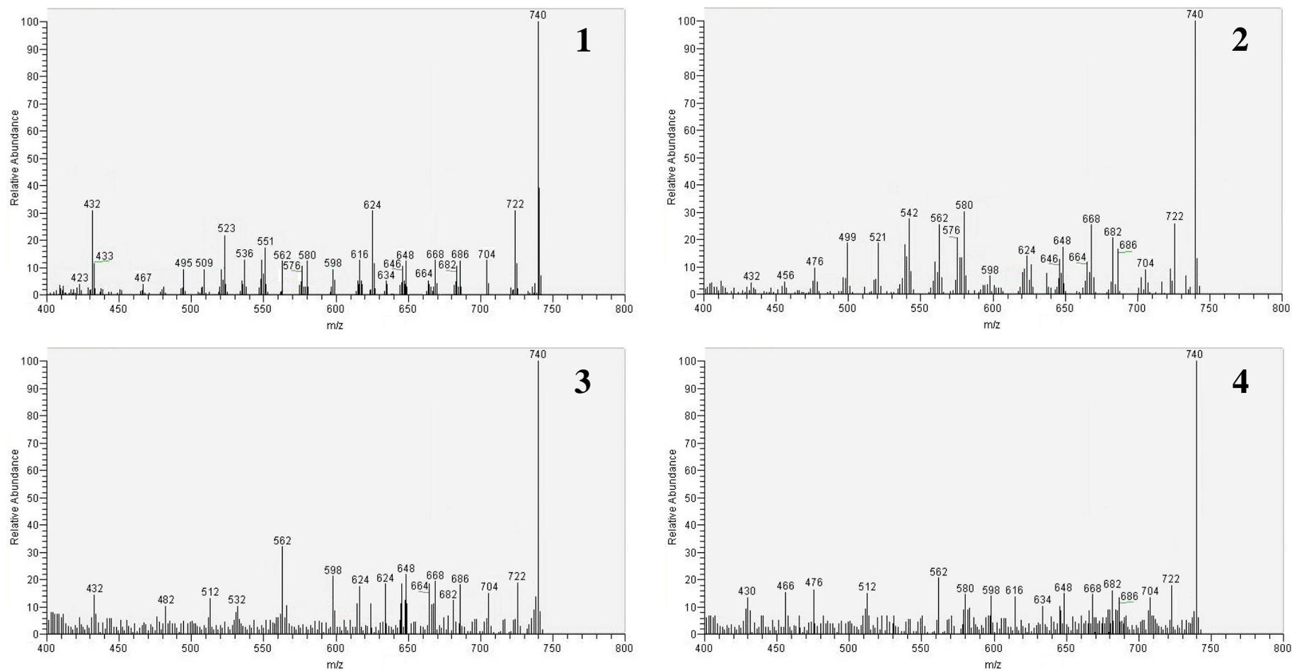
**Figure 16.** Mass spectra (EI mode) of major carotenoids fractions at retention of 15.17 min (1), 15.84 min (2), 16.40 min (3), and 16.88 min (4) separated by an Inertsil ODS-3 C<sub>18</sub> reversed-phase column (4.6 mm × 250 mm).
