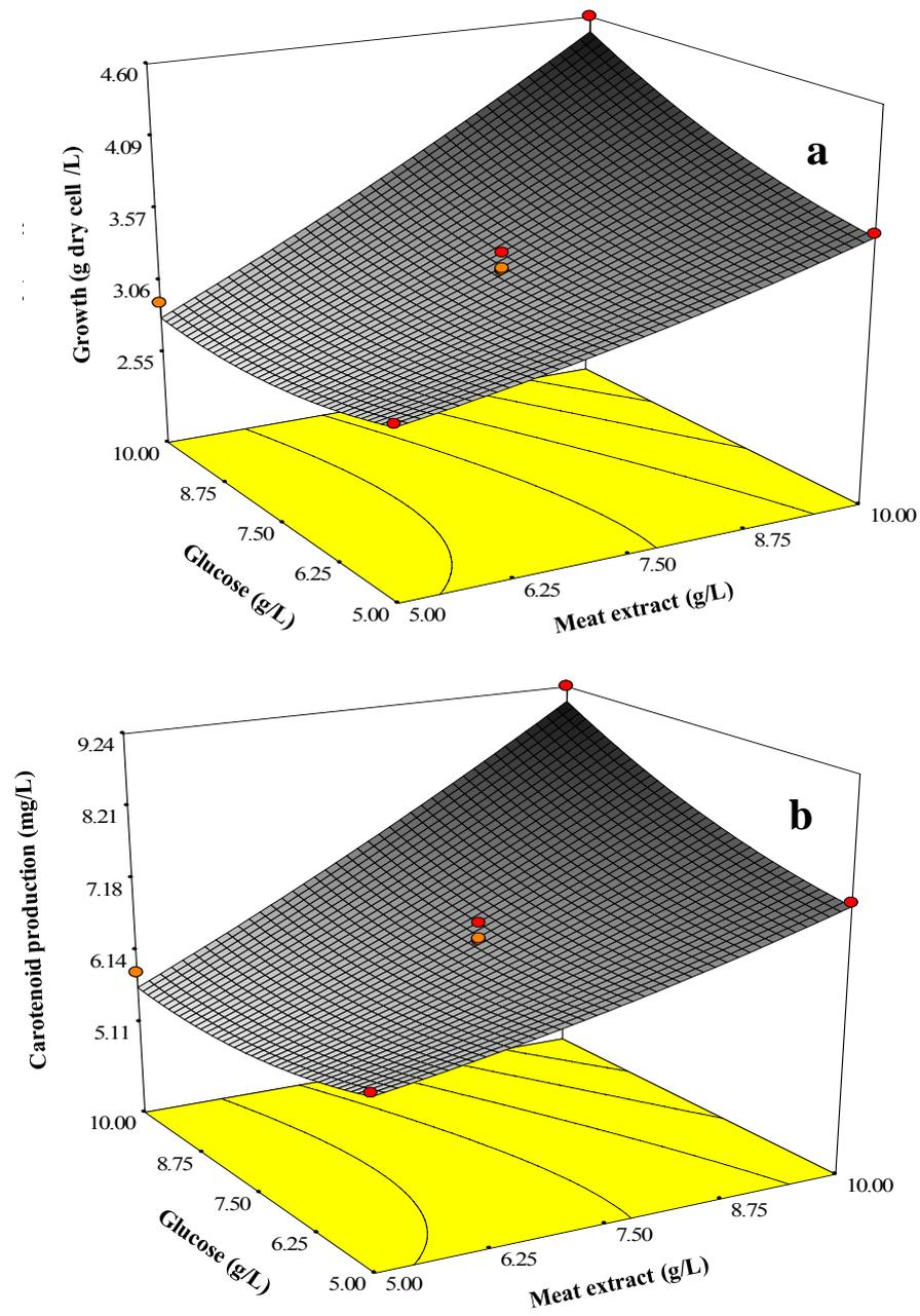
**Figure 19.** Three-dimensional response plot showing the effect of meat extract and glucose on growth (a) and carotenoid production (b).
