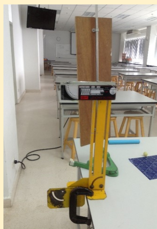
Figure 3.5b: Spring gun shooting of the projectile with the same initial velocity
