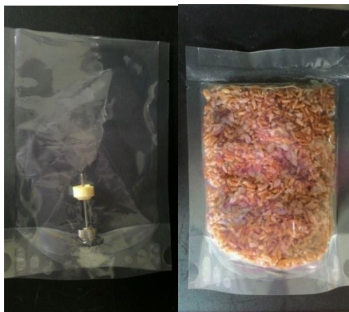
Appendix Figure 11 Retort pouch was inserted probe at the half of its height
