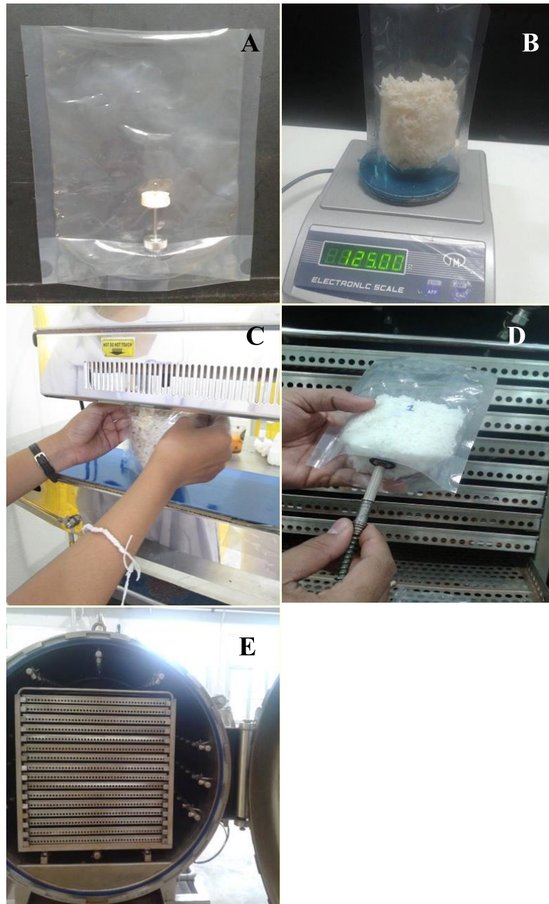
Appendix Figure 10 Monitoring of heating process time ( F_0 ) of cooked rice in a retort pouch, inserting thermometer needle into a retort pouch (A), sample weighting (B), sample sealing (C), thermocouple connection with computer for recording temperature (D) and sample loading into a retort (E)
