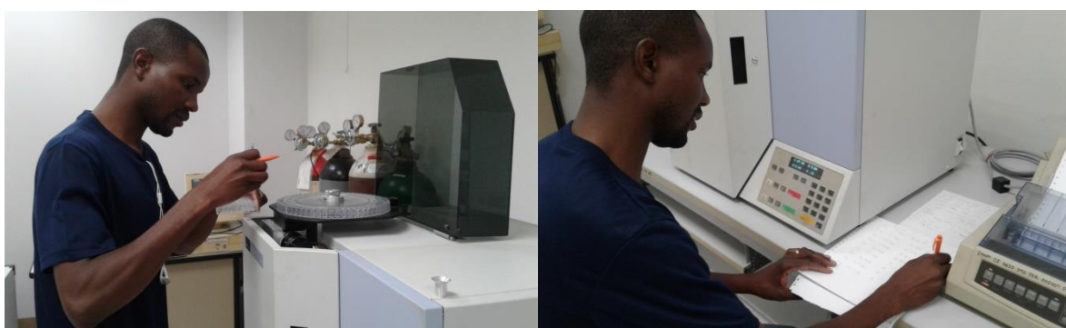
Plate D6: Elemental analysis using the 2400 Series II organic Element Analyzer (Perkin Elmer)
