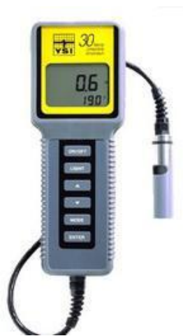
Figure 3.3 YSI Model Y30 SCT to measure salinity.
