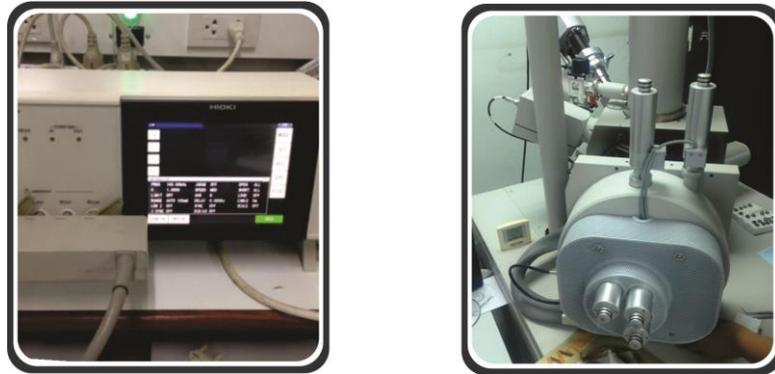
Fig. 2 LCR meter and Scanning Electron Microscopy
