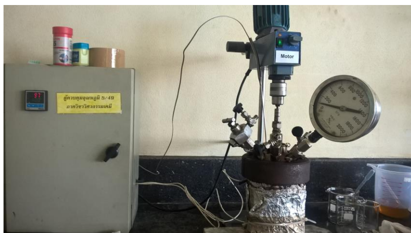
Fig. 6 The high pressure apparatus for the second stage transesterification.
