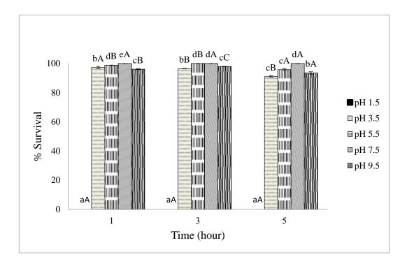
Supplemental figure 4 Stability of phage powder at various pH (trehalose alone).
