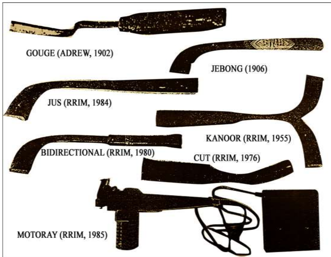
Figure 2 Development of tapping knives in Malaysia
