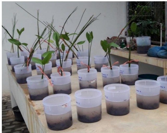
Figure A-2 Experimental set up for selected aquatic plants: Echinodorus cordifolius and Lepironia articulata with five replicates with controls.
