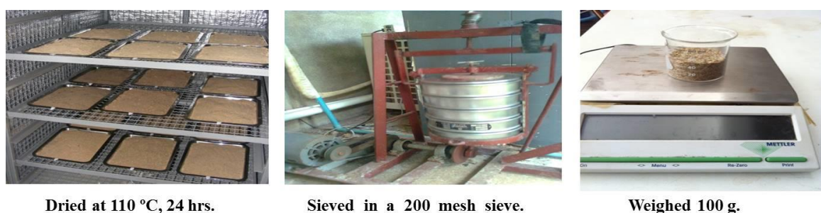
Figure 3.11 The soil sample sample preparation for measurements of effective radium content.
