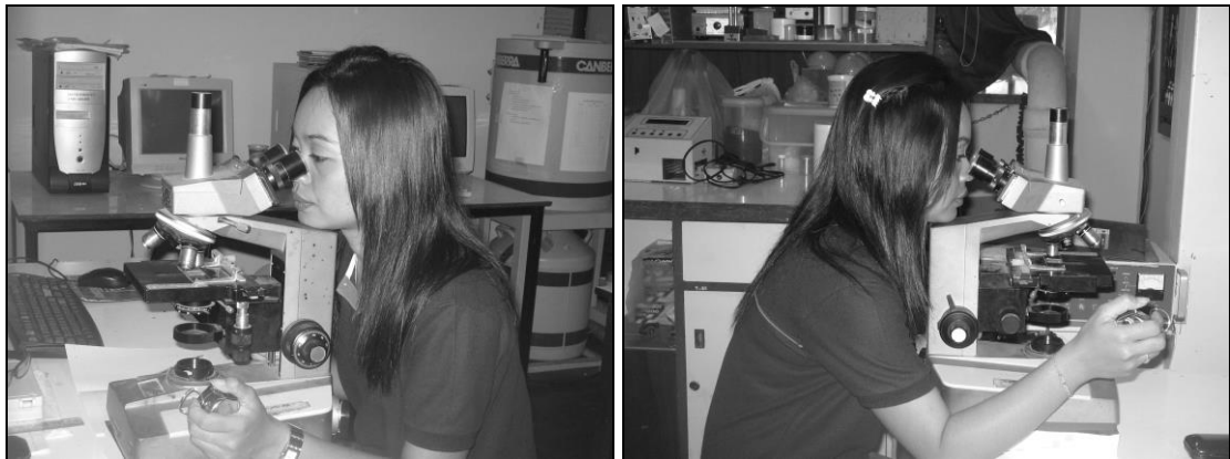
Figure A1.3 Counting tracks by using an optical microscope (OLYMPUS-BHC) at magnifications 10 \times 10 ( \times 100 ).
