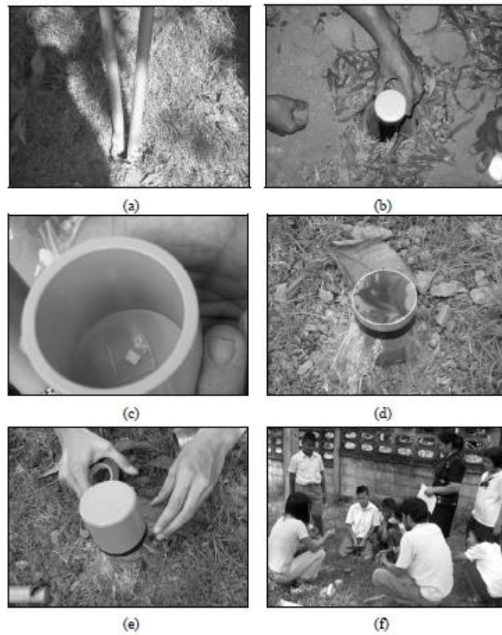
Figure 3.5 The measurement method of track detector for radon in soil gas: (a) a hole of 1 m depth, (b) a plastic tube put into the hole, (c) the tube was covered with thin polyethylene film and sealed airtight by a standard electrical tape, (d) the CR-39 film in a lid, (e) cover tube lid down and sealed airtight by a standard electrical tape, and (f) CR-39 film was changed every week.
