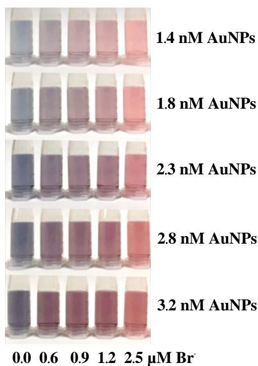
Figure A8 The color of solution on the effect of concentration of AuNPs corresponding to the linearity curve of \text{Br}^- concentration ranged from 0.63 - 2.50 \mu\text{M} \text{Br}^- (Figure A5).
