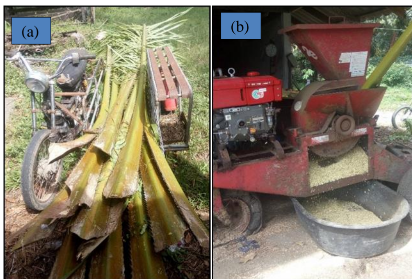
Figure 3.5 Oil palm frond stems chopping by Cutting-Machine
