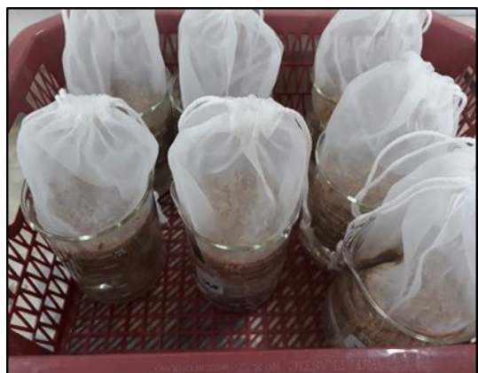
Picture 22. Filling sample into nylon socks with deionized water for bulk density
