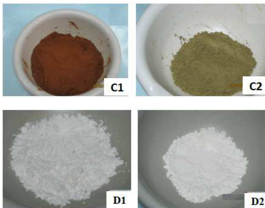
Fig.1. The precursors prepared by the co-precipitation method and perovskite oxides after being calcined at 900 °C for 2 h : A1) \text{LaAlO}_3 precursor, A2) \text{LaAlO}_3 perovskite, B1) \text{LaCoO}_3 precursor, B2) \text{LaCoO}_3 perovskite, C1) \text{LaFeO}_3 precursor, C2) \text{LaFeO}_3 perovskite, D1) \text{LaGdO}_3 precursor, D2) \text{LaGdO}_3 perovskite at 1200 °C.
