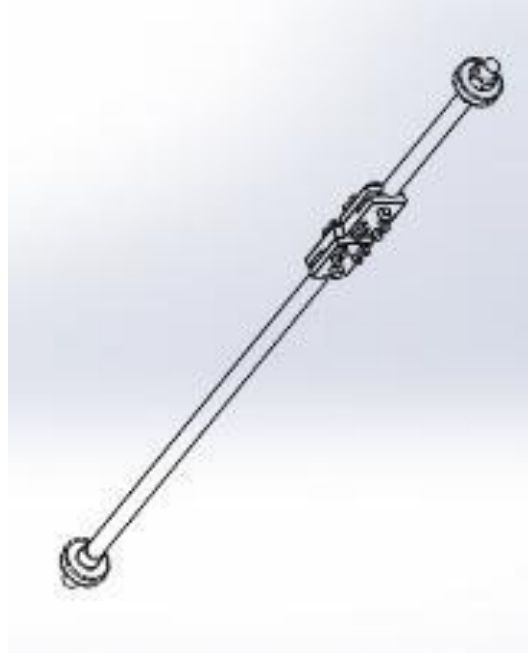
Fig. 19. The extensometer and holder system.
