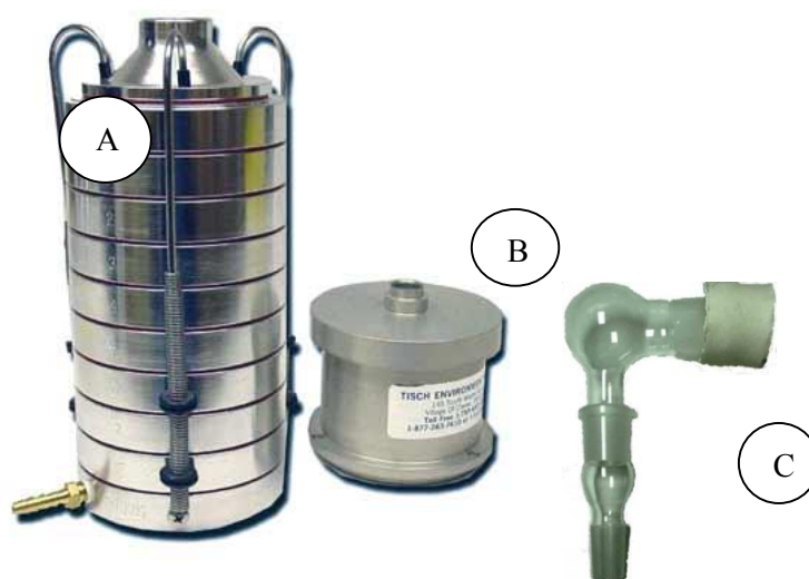
Figure 2 Eight stages Mark II Andersen cascade impactor (A), preseparator (B) and the glass throat (C) induction port
