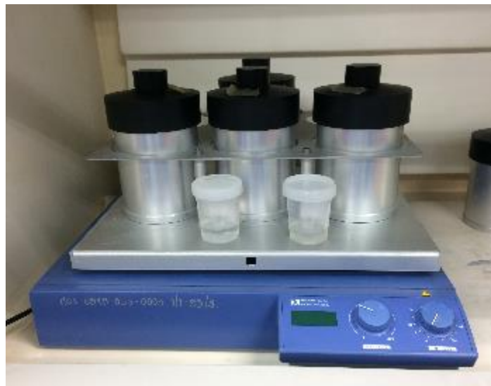
Figure 15: The specimens were dehydrated using ascending grades of alcohol, infiltrated and embedded in MMA
