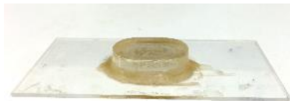
Figure16: The specimens were embedded in MMA and completed polymerization for undecalcified sectioning
